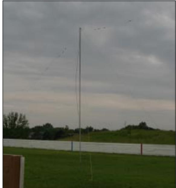
The hockey rink provides a great location for the multiband dipole antenna.
