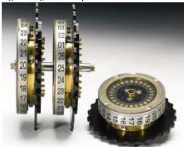
These are three of the rotors the operator changes to modify the message coding.
