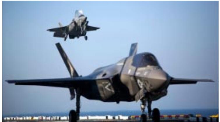
Two F-35B Lightning II Joint Strike Fighters complete vertical landings aboard the USS Wasp (LHD-1) during the opening day of the first session of operational testing.
