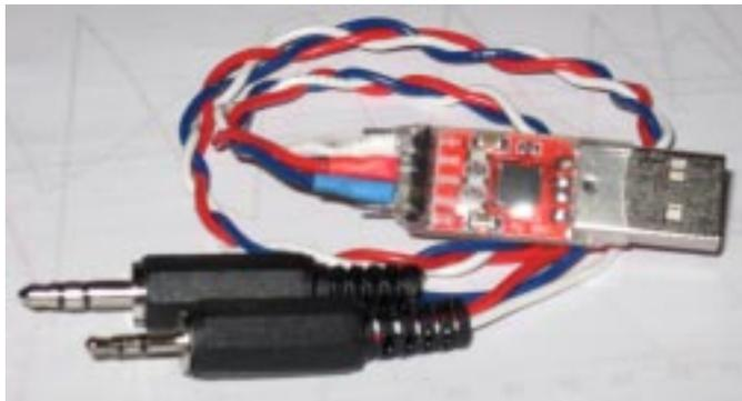
You will have to plug in the soldering iron and make three connections: TX Data (Blue), RX Data (Red), and Gnd (White). The connections to the plugs are wired like this picture.
