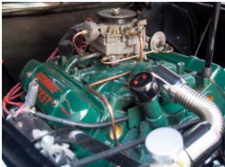
The Batmobile’s engine, Olds 88 324CID, 200HP Rocket engine was also restored
