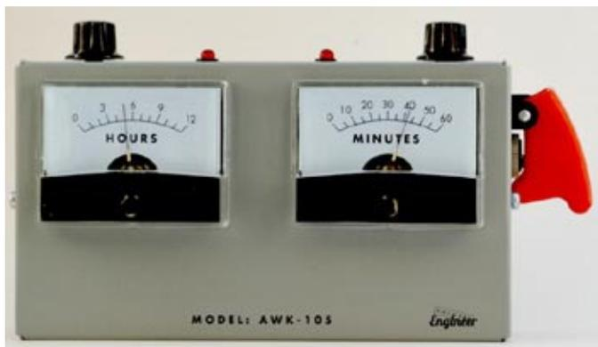
The device also features a custom-designed Atmel ATtiny microcontroller-based circuit board, an AM/PM indicator LED, an optional backlight on its display, and mode-select knobs on top. It's powered by a USB cable, which can be plugged into a conventional outlet using an included "wall wart" adapter.
