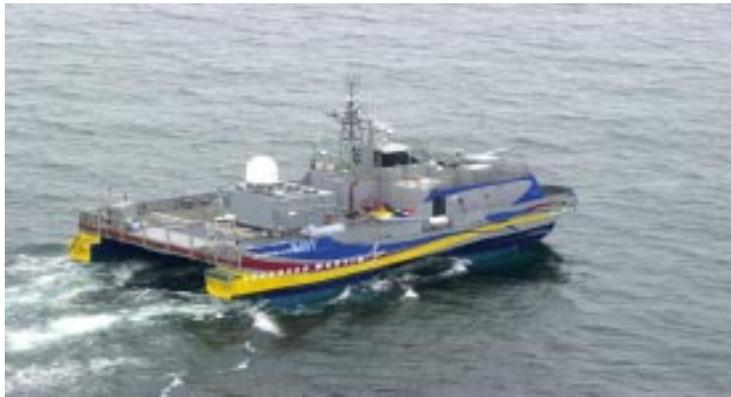
The 105-ft (32-m) long, 55-ft (17-m) wide, 180-ton (163-tonne) watercraft features two 3,480 hp diesel engines, two 180-kW Caterpillar diesel electric generators, and (if its specs are still the same as they were when it was first built) a top speed of 30 knots (56 km/h, or 35 mph). There's no word on how many people it can accommodate, although judging by the photos, there are at least six bunks. It also has a full galley, shower-equipped bathroom, plus a washer and dryer.
