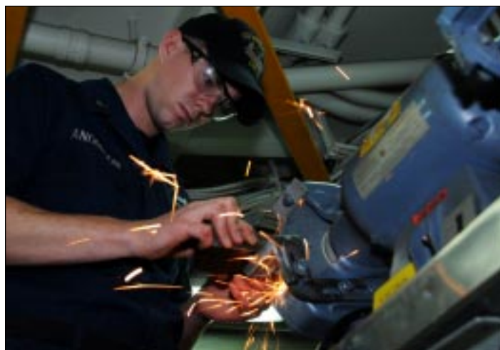
PACIFIC OCEAN Machinery Repairman 2nd Class Jared C. Anderson, from Anoka, Minn., grinds a grooving tool bit in the machine shop aboard the aircraft carrier USS Ronald Reagan (CVN 76). Ronald Reagan is underway conducting operations in preparation for an upcoming deployment.
