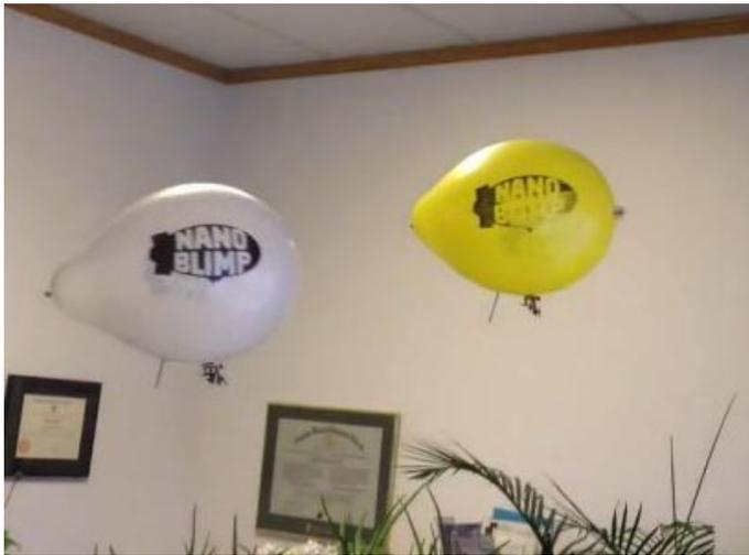
Users control the blimp via two joysticks on the included 3-channel Nano-X controller, which doubles as the charger for the gondola motors. It can be set to any of four different radio frequencies, which allows multiple Nanoblimps to be flown in the same room without interference. As can be seen in the video below, this makes it possible to engage in aerial dogfights, in which thumbtack-equipped blimps attempt to pop one another.
