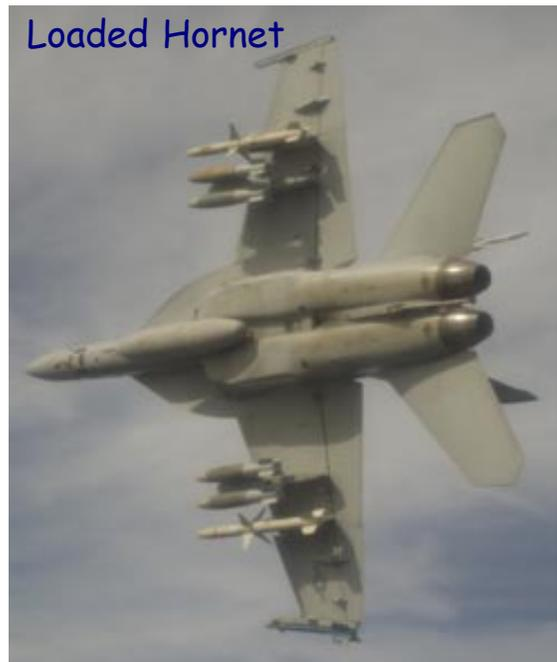
PATUXENT RIVER, Md. An F/A-18F Super Hornet assigned to the Salty Dogs of Air Test and Evaluation Squadron (VX) 23 conducts a captive carry flight test of an AGM-88E Advanced Anti-Radiation Guided Missile (AARGM) at Naval Air Station Patuxent River, Md.
