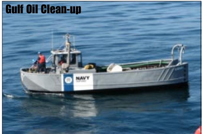
A rapid-deployment skimmer system, operated by Naval Sea Systems Command's Supervisor of Salvage and Diving (SUPSALV), as it conducts oil spill response training. The Navy sent 66,000 feet of inflatable oil boom, skimming systems, related support equipment and personnel to support clean-up efforts for the Deepwater Horizon oil spill on April 28<sup>th</sup>
