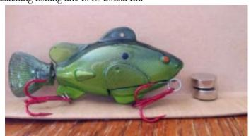
An integrated sensor activates the lure as soon as it enters the water. This causes its two electromagnets (one on either side of the fish) to alternately turn on and off in quick succession. This in turn causes a third magnet, located between the two, to be drawn back and forth from one to the other. That magnet is joined by a shaft to the tail, so the ultimate result is a flapping tail that propels the lure forward in a "fish-like" manner.
