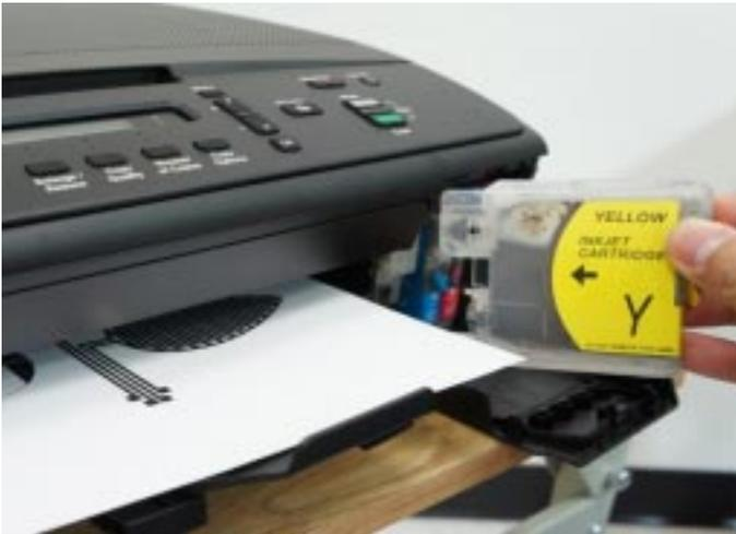
Silver nanoparticle ink is injected into ink cartridges for an off-the-shelf printer to create cheap, foldable circuitry
