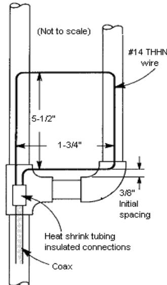
Adjusting the loop for minimum SWR is simple: Move the loop up or down from its initial position until you find the point of minimum feed-line SWR. Once you've found this point, secure the loop as closely to the J's copper pipe as possible with nylon tie wraps.
