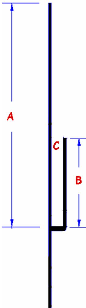
The dimension for the parts of the J-pole are, the 3/4 wave vertical, dimension A, 58", the 1/4 wave stub 19 1/4", the center-to-center spacing between the two verticals, dimension C, is 1 3/4" inches. Since the actual fittings vary, you will have to determine the length of the short pipe between the Tee and regular El fittings to produce the 1 3/4" center-to-center spacing of the elements. Fire up your propane torch and solder all pipe joints.
