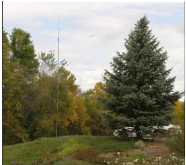
The site layout for the event resulted in a three story building between the radio communications table and the stations on the course. The solution was a J-pole on a 25 foot mast (on the left above) driven by a mobile transceiver (in white car behind pine tree) cross-banding with a HT from the NECOS location. (W0NFE photo)
