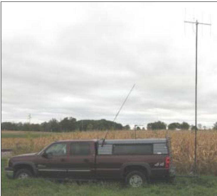
The Lima 2 antenna farm was made up of Dan's, N0PI, hitch mounted portable mast supporting a 4 element yagi. Dan crossbanded to the transceiver installed in the truck. (N0PI photo)
