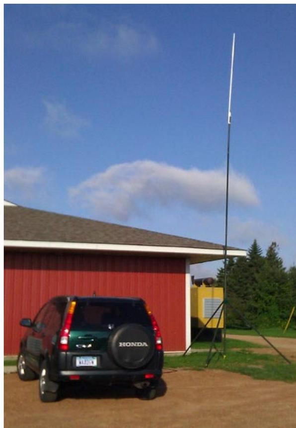
John, WA0DGW used a GoVertical approach to get a good signal from the farthest point on the route to the NECOS. Crossbanding with an HT to the Dualband Xcvr in the vehicle and the elevated antenna did the trick. (WA0DGW photo)
