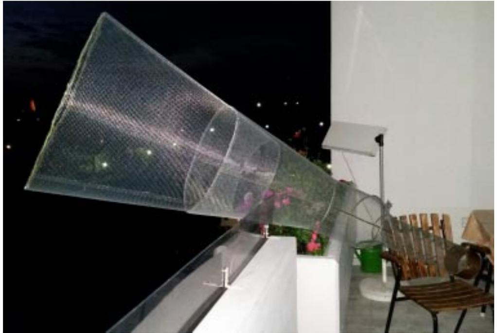
The Moonbounce antenna used was a W2IMU feed made of 6mm mesh by adding a large cone, achieving a horn antenna with 80cm mouth diameter. Estimated gain is 19dBi, maybe slightly less. Shown here on the balcony pointed at the moon.
