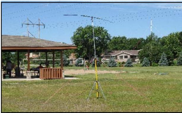
A number of antennas were tested by ARES members during the Field Day event. Pictured here are a Buddi Pole dipole (foreground) and a multiband dipole (background right). Other antennas tested included a ‘slinky’ dipole and several VHF antennas.
