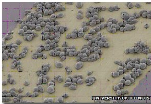
Tests showed small microcapsules filled with liquid metal healed fractures in a gold circuit restoring conductivity
