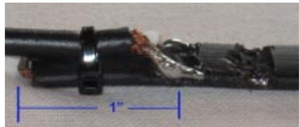
The feedpoint connection of the coax. A tie-wrap serves as a strain relief. The feedpoint is about 6-7% of the length of the stub from the shorted end.
