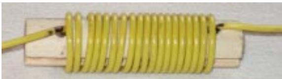
Coil wound on a 1/2" diam. wood dowel. Note the position of the sharpie length markings on the coiled wire.
