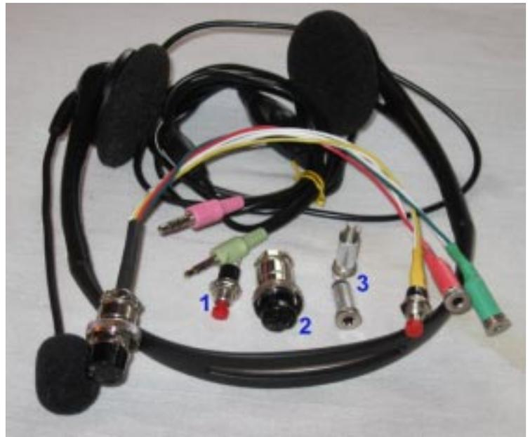
Once you find your economical headset all you need is 1.SPST NO pushbutton switch, 2.Mic connector to match your radio, 3.two in-line 3.5mm stereo jacks. You can class up the connections with some color coded heat shrink tubing.
