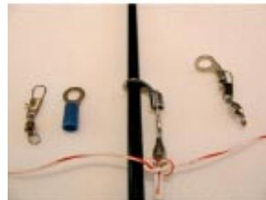
above shows how to make a simple centre support using a fishing snap swivel and a crimp ring terminal. The bottom of the snap swivel is at the centre of a "Electricians Knot" used to tie the two halves of the wire doublet together. I can't take credit for coming up with this idea (it came from someone on QRP-L) but I have used it a lot and it works very well.
